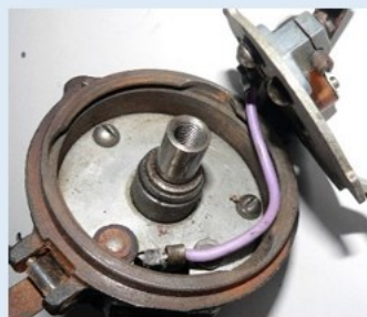
The condenser, which is prone to heat, can be mounted on the upper plate.
