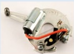
The condenser, which is prone to heat, can be mounted on the upper plate.
